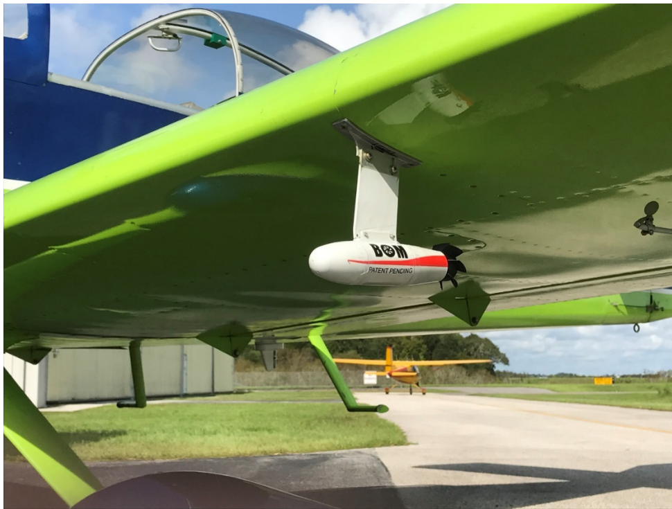
Fig 6. BOM installation on an RV9 using an external bracket. Notice the pitot on the right is at the same distance from the wing
