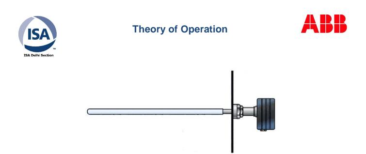
Flyash particles passing near the electrodynamic probe induce a small voltage in the probe. The frequency of this signal is analyzed to determine the flyash loading.
