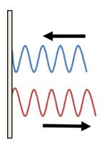
Typically, the reflected signal is out of phase with the transmitted signal. This causes the signals to decay quickly keeping the energy level low.
