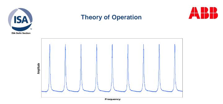
The frequency of the transmitted signal is varied across a 100MHz range. Whenever a resonance is encountered, a peak occurs. The amplitude of the peaks decrease in proportion to the amount of carbon in the backpass.
