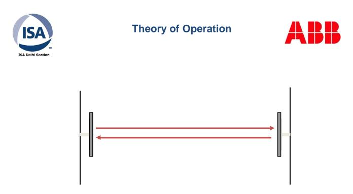
To increase the sensitivity to carbon, the signal can be reflected back and forth many times.
