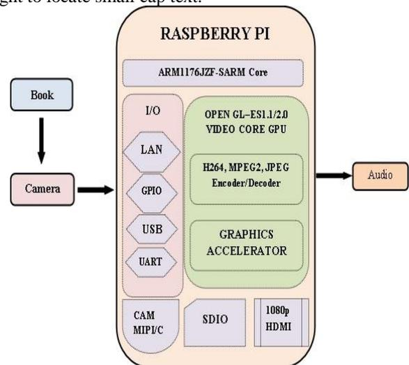
Fig.1: system architecture for product label reading
