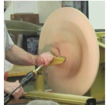
Using a gouge to hollow out a depression. Can also use scrapers as needed.
