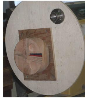
"fixing" board is secured on wooden faceplate and assembly is checked for balance
