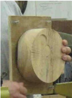
Demo blank on "fixing" board
