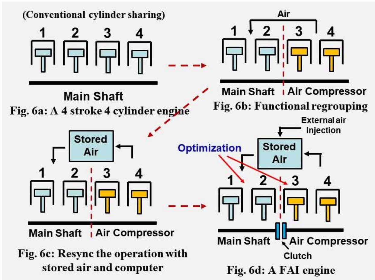
**Fig. 6: Evolution from a conventional four-stroke engine to a two-stroke FAI engine**
