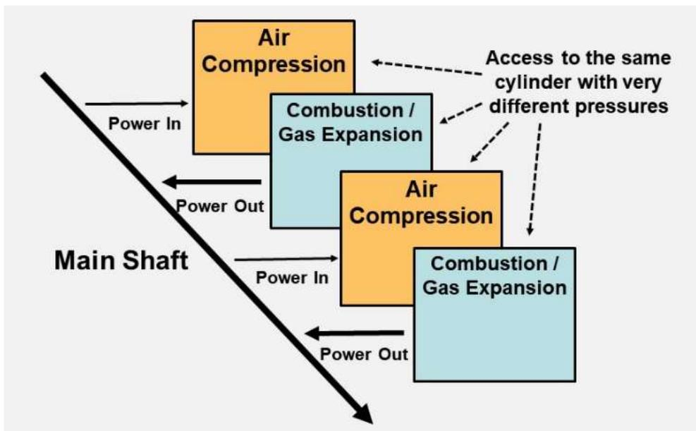
**Fig. 4: A conventional cylinder sharing engine structure**
