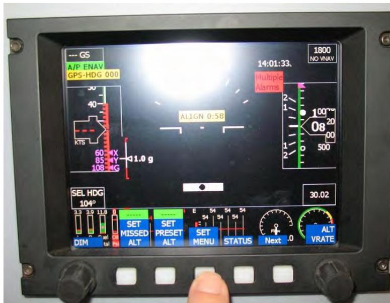
This will bring you to the Settings Menu. Once there, rotate the right knob until the box is around Display Unit Maintenance. Press the right knob to select Display Unit Maintenance.
