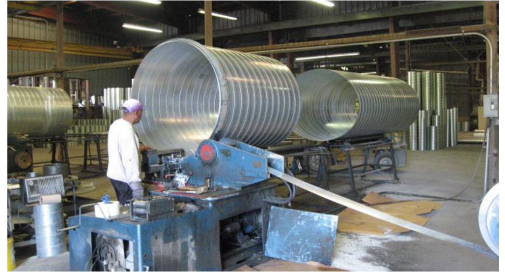
Round duct and its child, “flat oval” are made on a spool coil machine.
