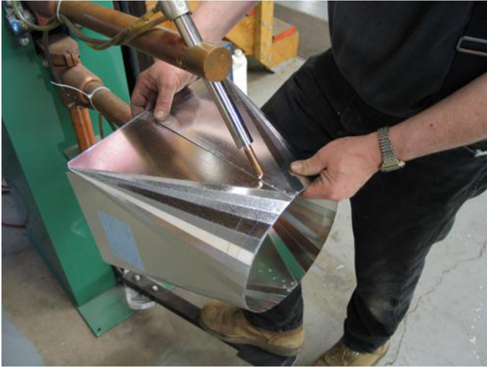
Fitting hand-labor. Tack-welding a transition.
