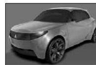
A lithium-ion powered hybrid concept vehicle, the Concept-CT MIEV, featuring four electric wheel motors, was unveiled by Mitsubishi at the Detroit Auto Show. Unlike
