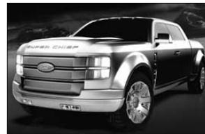
Ford showed several energy-conscious concept vehicles at the Detroit show, including the F250 Super Chief, a tri-fuel (gasoline, E85 and hydrogen) truck, which boasts a V-10 engine that puts out 400 lb.-ft. of torque running on hydrogen.
