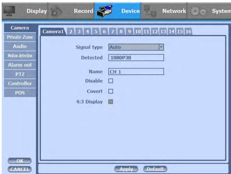
\* The figure above shows that the camera is 1080P 30fps (NTSC).
