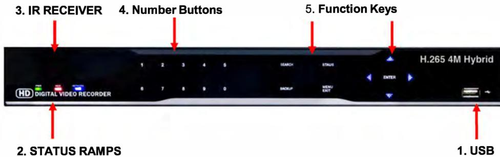
1. **USB** : These USB ports are for mouse and USB devices. You should connect correctly the USB devices and mouse as picture directed.
