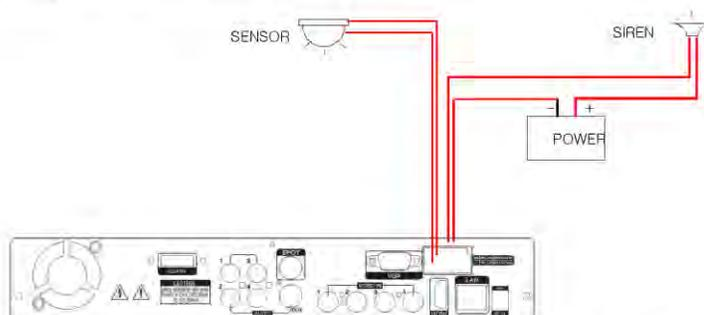
**Sensor In :** Connect the sensors. The sensor are composed of both signal and ground terminals, with a voltage difference of 5V. In the case that the sensor used for input is of the N/O (Normal Open) type, when the voltage difference between the signal and ground falls to 0V (short), the DVR can use this as a trigger to start alarm/sensor based recording.
