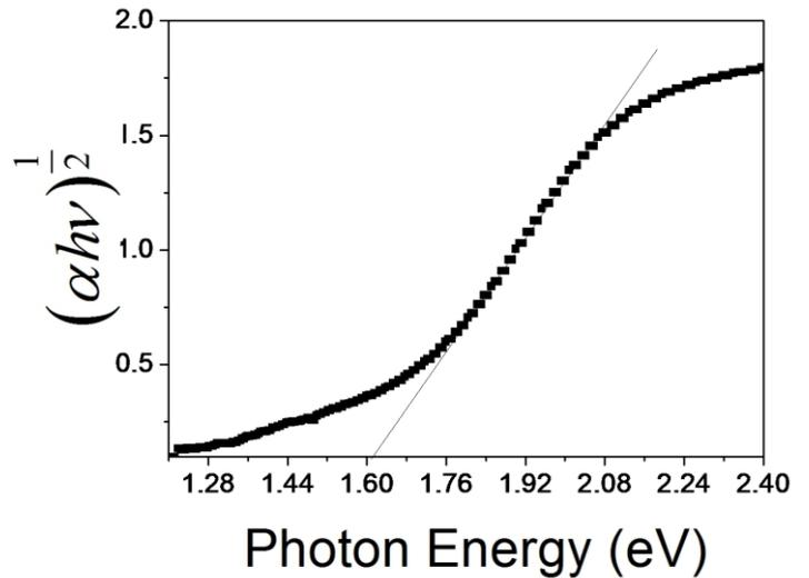
Fig. 5. Tauc's plot obtained from UV-vis spectrometry showing  $(\alpha hv)^{\frac{1}{2}}$  vs  $hv$  graph.
