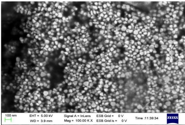
Fig. 3. SEM of synthesized CdS nanoparticles with X = 100 K.
