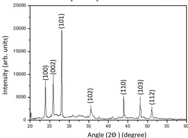
1. XRD pattern of synthesized CdS nanoparticles.
