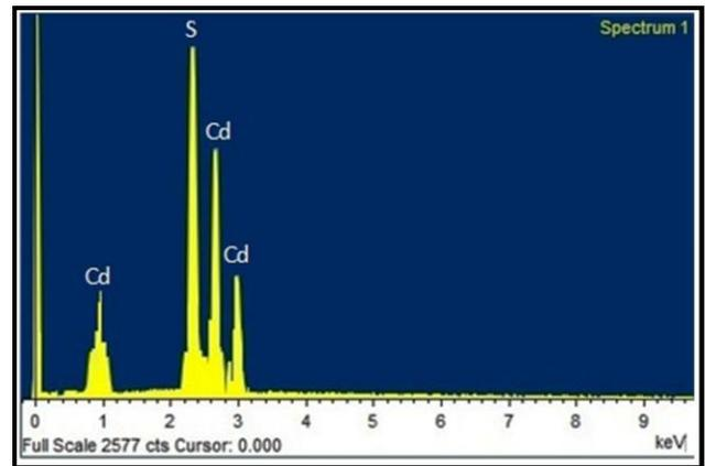
Fig. 2. The elemental compositions of the synthesized CdS nanoparticles observed by EDS
