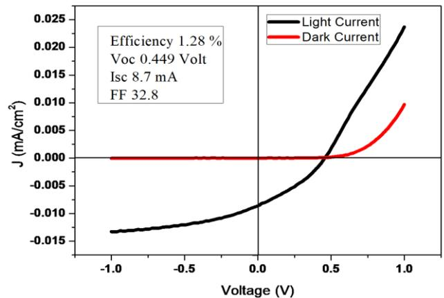
Fig. 6. J-V characteristics of fabricated glass/ITO/CdS/Al solar cell device measured under dark and illumination.
