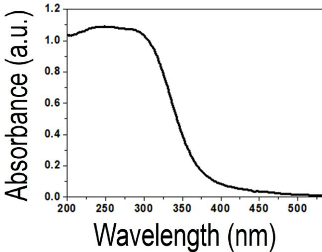
Fig. 4. UV-vis absorption spectra of CdS nanoparticles.
