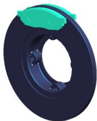
Fig.2 Simplified Disc & Pad Assembly
