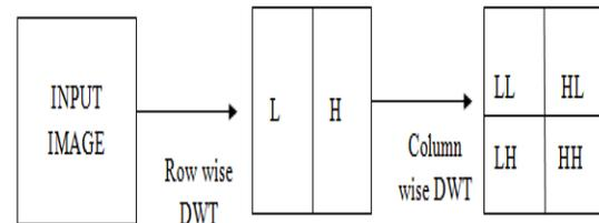
Fig.1: DWT Operation on Image
