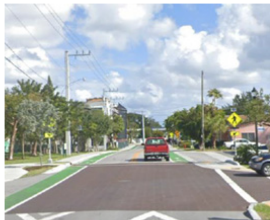
Typical raised intersection installed in Fort Lauderdale
