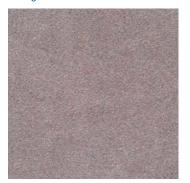
C HB21/2 Rust grade C Hydroblasted to an Sa21/2 equivalent
