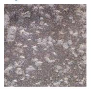
D HB21/2 Rust grade D Hydroblasted to an Sa21/2 equivalent
