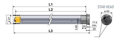
2 mounting holes for self tapping screws. Dia. 5 mm (cat #9670013). Depth 13 mm spaced 1.89" (48 mm) apar
