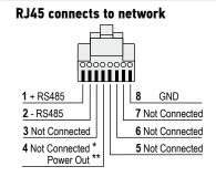
4 Cond. 26AWG modular cable with RJ9 on one end and RJ45 other end - (RTS, Z-Wave®, ZigBee modules)
