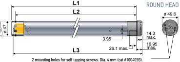
2 mounting holes for self tapping screws. Dia. 4 mm (cat #100405B). Depth 9 mm spaced 1.14" (29 mm) apart.
