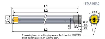
**Dimensions** 506S2PA 506S2PS\*\* 510S2PA 510S2PS\*\* L1 23.74 in. (603 mm) 23.74 in. (603 mm) 23.74 in. (603 mm) 23.74 in. (603 mm) L2 23.23 in. (590 mm) 23.23 in. (590 mm) 23.23 in. (590 mm) 23.23 in. (590 mm) L3 24.25 in. (616 mm) 24.25 in. (616 mm) 24.25 in. (616 mm) 24.25 in. (616 mm) Cable Length 5 in. (.12 m) 5 in. (.12 m) 5 in. (.12 m) 5 in. (.12 m)
