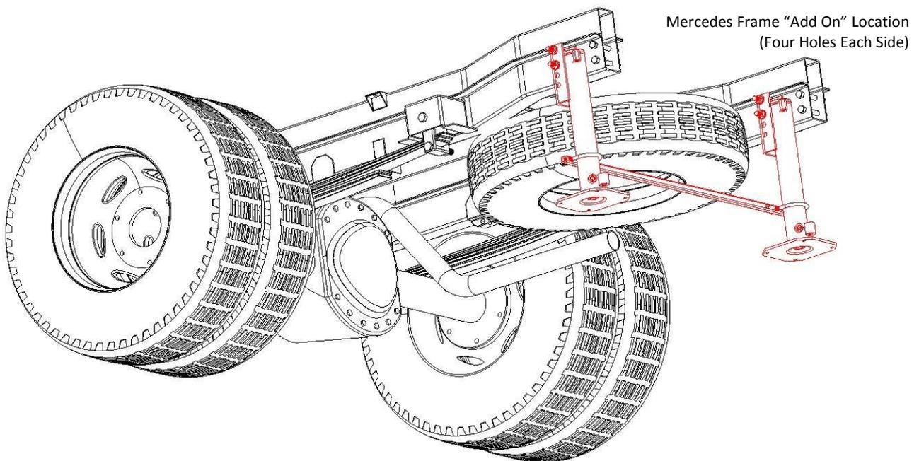
Remove old hardware (two bolts per side), Mount jacks utilizing existing holes by utilizing included longer hardware (1/2" Grade-8 6 1/2" Bolts & Flange Lock Nuts). Crossbrace is required.
