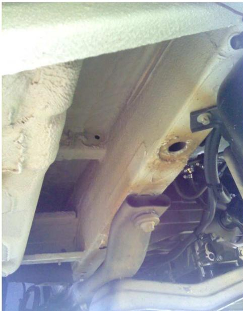
Passenger side jack location (under cab) cylinder also mounted on the outside face of the frame. Removal of the storage box in the step rail (shown in picture) must be removed. Angle drill will be required for 5/8" or 3/4" hardware.
