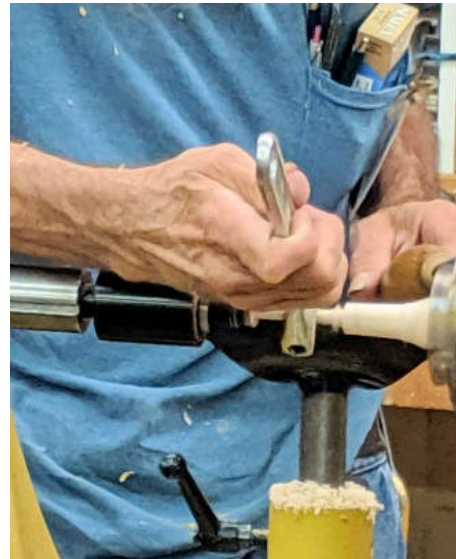
Ian uses a wrench to measure the diameter of the stem to make sure it will slide easily inside the ring of the top.
