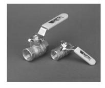
sure areas of the piping system.) Brass lever-handle ball valves supplied by **OmegaFlex**® are rated for 5 PSI use and are available in 1/2 inch and 3/4 inch sizes.
