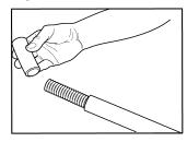
5. Using a twisting motion, remove the black sleeve from the pipe. It may be necessary to cut sleeve longitudinally and peel off for larger sizes. <u>Inspect stainless pipe for</u> <u>scoring from the tubing cutter.</u>
