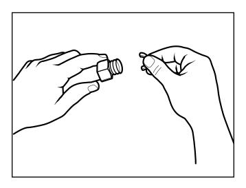
3. INSTALL FITTING NUT: Slide nut over cut end: place two split-rings into the first corrugation next to the tube cut. Slide nut forward to trap the rings.
