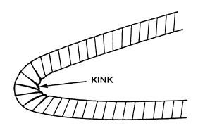
Figure: 5-3 – Repair Necessary.
