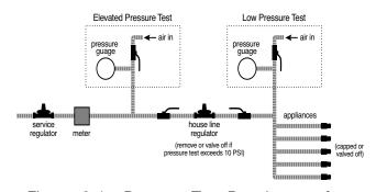
Figure: 6-1 – Pressure Test Requirement for a 2 PSI System
