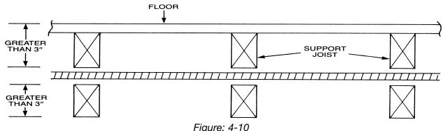
No Shielding Requirement at Support Area when Points of Penetration are greater than 3 inches from any Edge of a Stud, Joist, Plate, etc.
