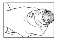
Holding the black coupling, slide fitting up to capture split rings into nut. Be sure split rings slip all the way to the base of the internal threads. Assembly is now ready to be attached to the adapter on the equipment.
