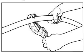
1. Unreel pipe into trench or on the ground and cut to desired length plus one additional foot. Cutting up to 1" size can be done with a large tubing cutter. For 1-1/4 to 2 inch sizes, a reciprocating saw is recommended.
