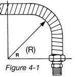
Multiple tight bends can restrict the gas flow and increase pressure drop. The tightest bend allowed for each size of **CounterStrike®** is shown in Table: 4-1.
