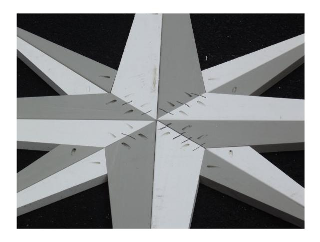
Screw your inlay together in pre-drilled pocket holes with screws provided, using plumbers PVC glue at the joints before final screws.
