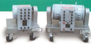
All machines are mounted on mobile bases and are equipped with either motor starter or circuit breaker protection.
