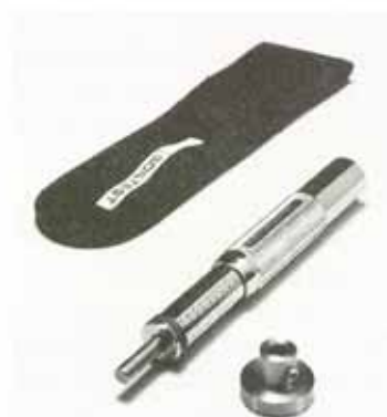
CL-700A penetrometer provides a relative indication of the compressive strength/density of lightweight insulating concrete. However, this test does not provide sufficient repeatable data nor the precision to use as a single source evaluation technique. (PHOTO COURTESY OF ELE INTERNATIONAL, INC./SOITEST PRODUCTS DIVISION, LAKE BLUFF, IL.)
