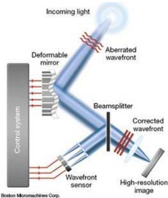
Figure 1. An adaptive optics system that diverts light from a distorted image via a beam splitter to the control system (computer) which controls a deformable mirror to correct the reflected image to match an idealized perfect star image model before reflecting the corrected image to the detector to the right.
