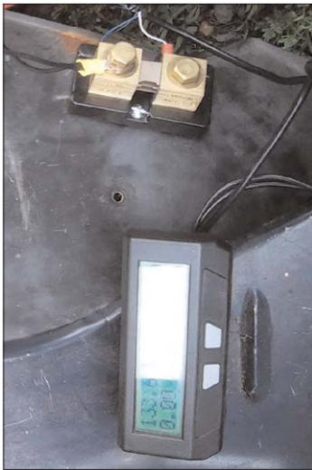
I also wanted to be able to get a read on the pack voltage digitally, and without closing the main contactor and making the vehicle live. I had an extra high current cycle analyst around (left, below meter shunt) that I wasn't using, and I wired that
