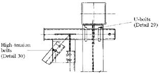
Beam-Column Connection for Truss Structure Example 18
