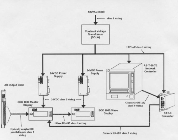
Class 1 wiring that is used with the SCC Display is the 120VAC power that is feeding the DC supplies, The NAB-3 converter and the AB T-60/70 controller. These should be fed from a constant voltage transformer. Class 1 wires can be run along with other class 1 wiring, but should not be run in close proximity to 220VAC or 440VAC wiring. Class 1 wires may be broken by any number of terminal strips or connectors, and require no shielding of the wires.
