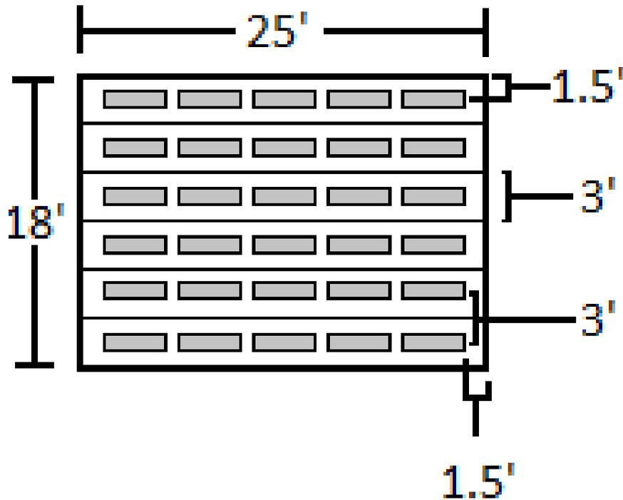
If designed as a conventional trench formation, the resulting footprint would be approximately 1,500 ft<sup>2</sup>. The above PPBPS bed formation offers a 70% reduction in area needed on the lot.
