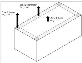
Illustration based upon ASCE 7-10, Fig. 30.4-2A ( $\theta \le 7^{\circ}$ ); Effective wind area = 10 ft<sup>2</sup>
