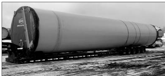
A section of the tubular support stand for a large wind generator
