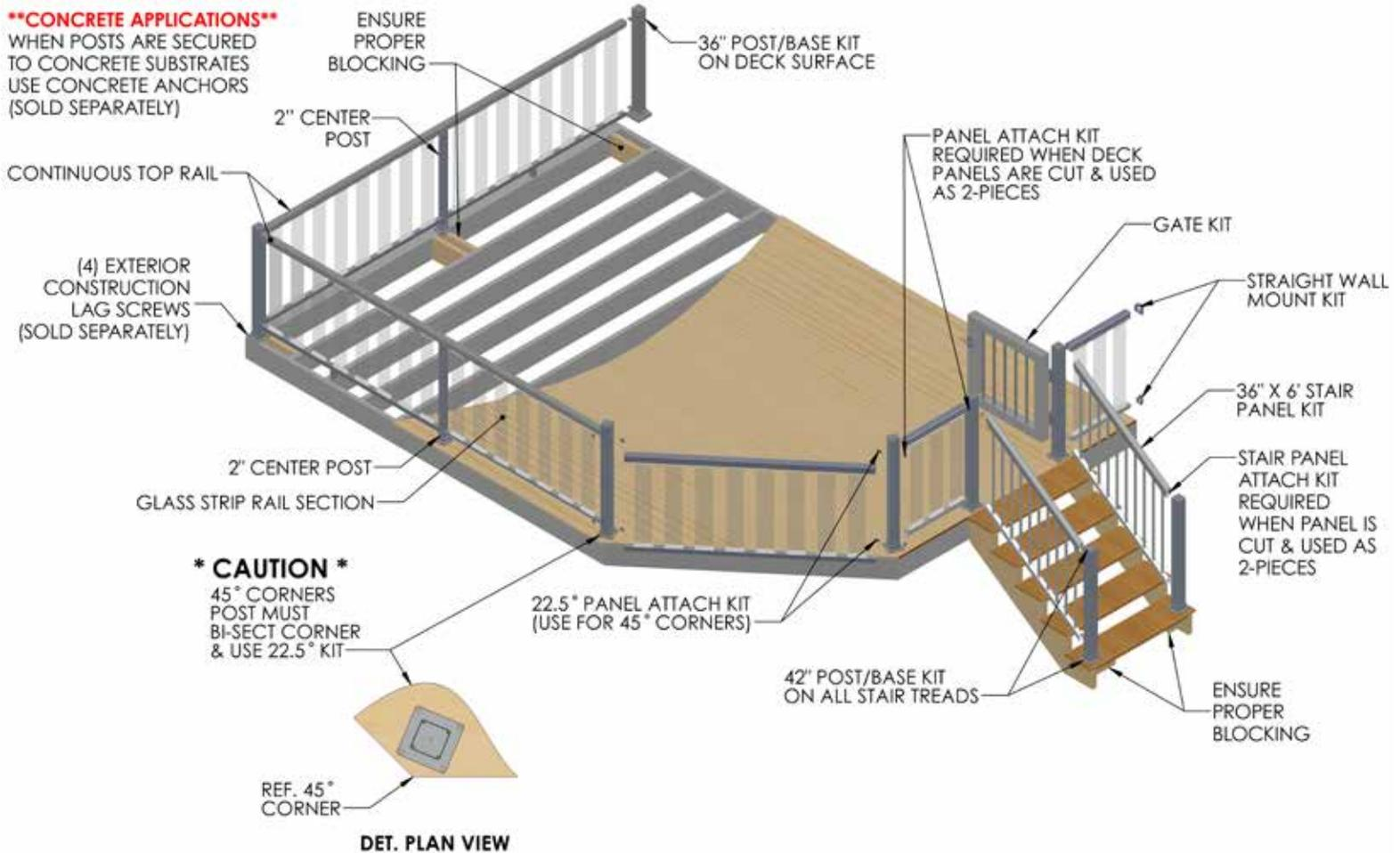
Prior to construction, check with your local regulatory agency for special code requirements in your area. Common railing height is 36" or 42". Never span posts more than 8' on center for picket railing systems and 6' on center for glass railing systems. Always ensure there is proper blocking under each post as per installation instructions. Read installation instructions and view installation videos to get a complete understanding of how the Harmony Railing™ products assemble.
