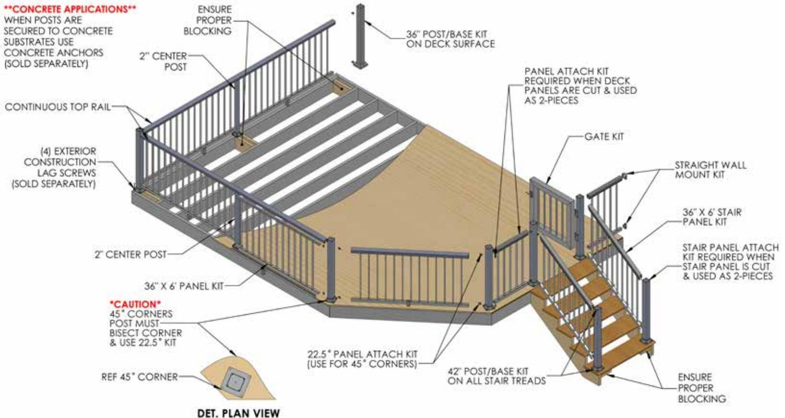
Prior to construction, check with your local regulatory agency for special code requirements in your area. Common railing height is 36" or 42". Never span posts more than 8' on center for picket railing systems and 6' on center for glass railing systems. Always ensure there is proper blocking under each post as per installation instructions. Read installation instructions and view installation videos to get a complete understanding of how the Harmony Railing™ products assemble.
