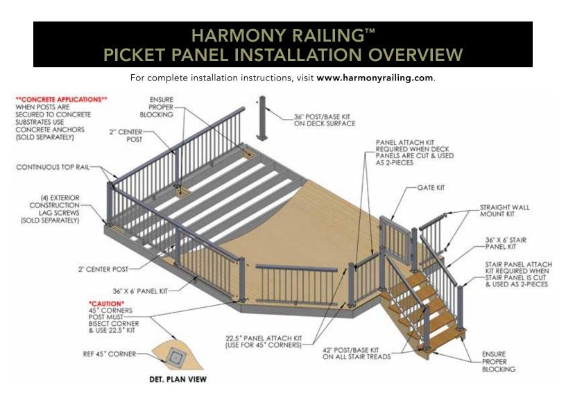
Prior to construction, check with your local regulatory agency for special code requirements in your area. Common railing height is 36" or 42". Never span posts more than 8' on center for picket railing systems and 6' on center for glass railing systems. Always ensure there is proper blocking under each post as per installation instructions. Read installation instructions and view installation videos to get a complete understanding of how the Harmony Railing<sup>™</sup> products assemble.
