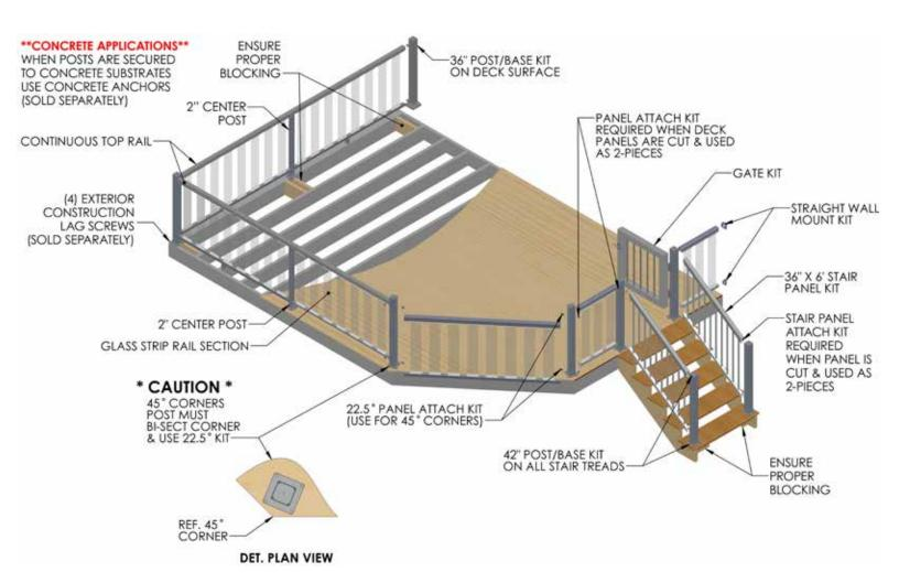
Prior to construction, check with your local regulatory agency for special code requirements in your area. Common railing height is 36" or 42". Never span posts more than 8' on center for picket railing systems and 6' on center for glass railing systems. Always ensure there is proper blocking under each post as per installation instructions. Read installation instructions and view installation videos to get a complete understanding of how the Harmony Railing<sup>™</sup> products assemble.
