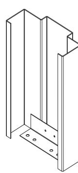
Masonry Base (Floor) Anchors
