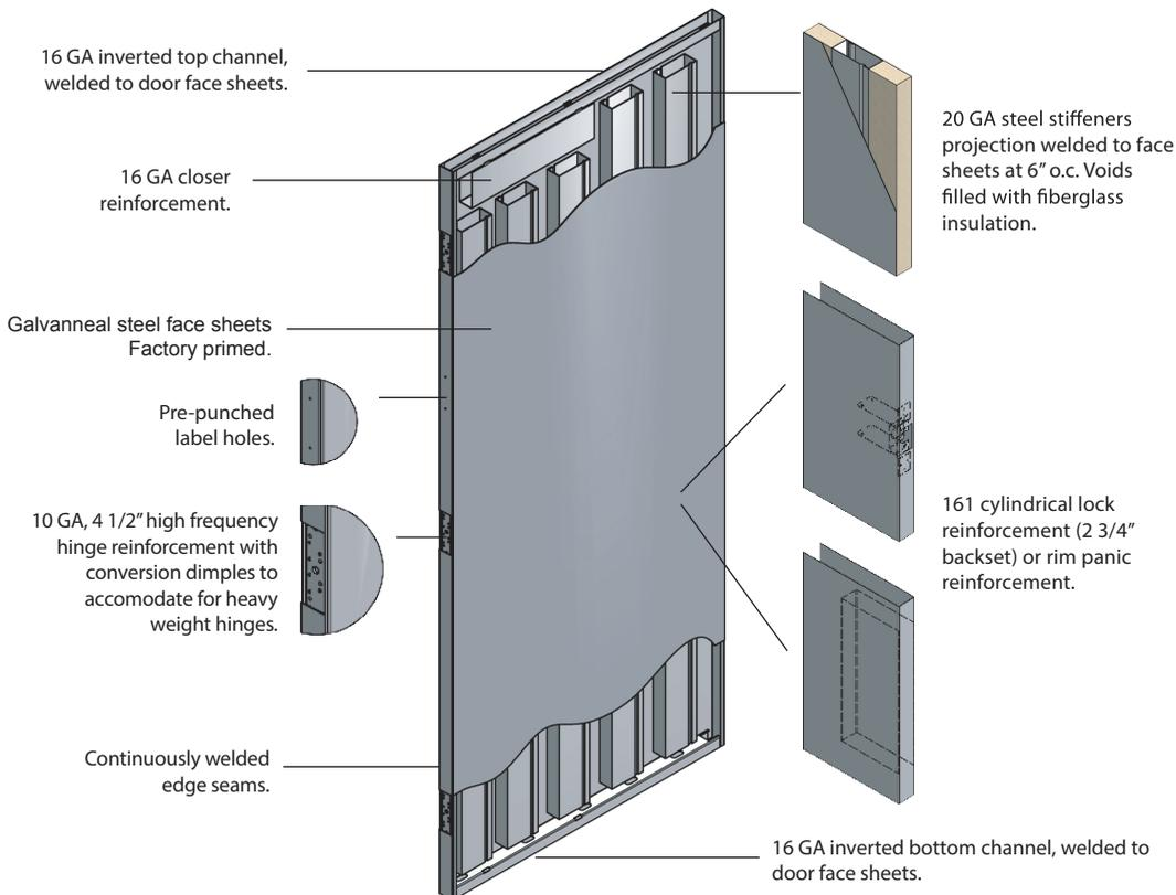
CW Series Doors are constructed with the purpose of providing the ultimate in strength and durability. With steel stiffeners welded to the door face sheets and edge seams continuously welded, CW Series Doors are the perfect solution for high security or high traffic areas such as schools and detention centers. CW Series Doors are available in 16 GA and 14 GA and can be fire rated up to 3 hours.
