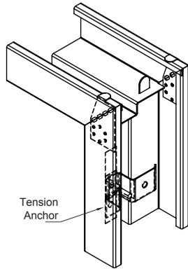
Typical KD (Knock Down) corner section includes tension anchor.
