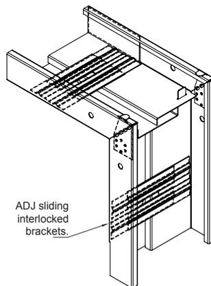
Typical KD (Knock Down) corner section includes sliding interlocked brackets.
