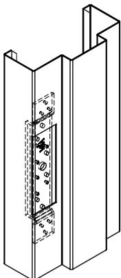
10 Gauge high frequency hinge reinforcing
