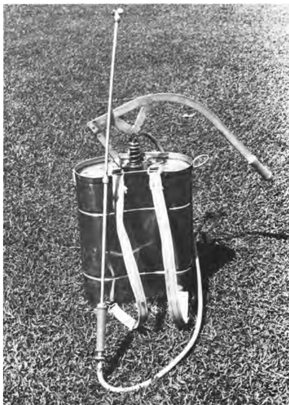
4.2 Top, a leverage-operated knapsack sprayer; bottom, a controlled-droplet applicator.
