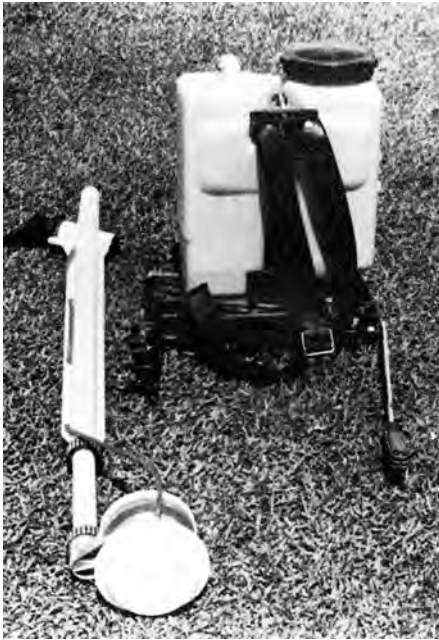
4.3 Controlled-droplet applicators that use a manually operated air pump are available.
