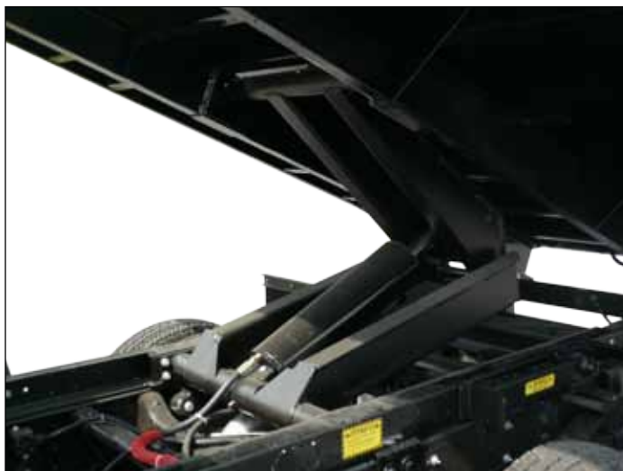
Hard chrome piston rod, lubricated bearing points, and full length subframe
