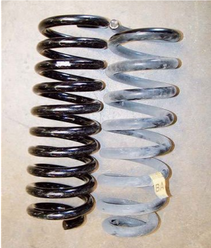
A spring compressor must be used to remove the spring from the strut. Note: After removing the spring, remove the plastic cap on the top of the strut, cut the foam bumpstop in half, and replace the cap.
