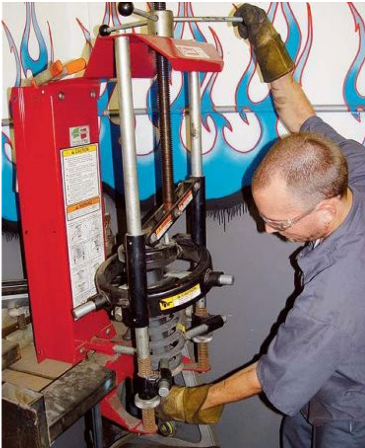
A spring compressor must be used to remove the spring from the strut. Note: After removing the spring, remove the plastic cap on the top of the strut, cut the foam bumpstop in half, and replace the cap.
