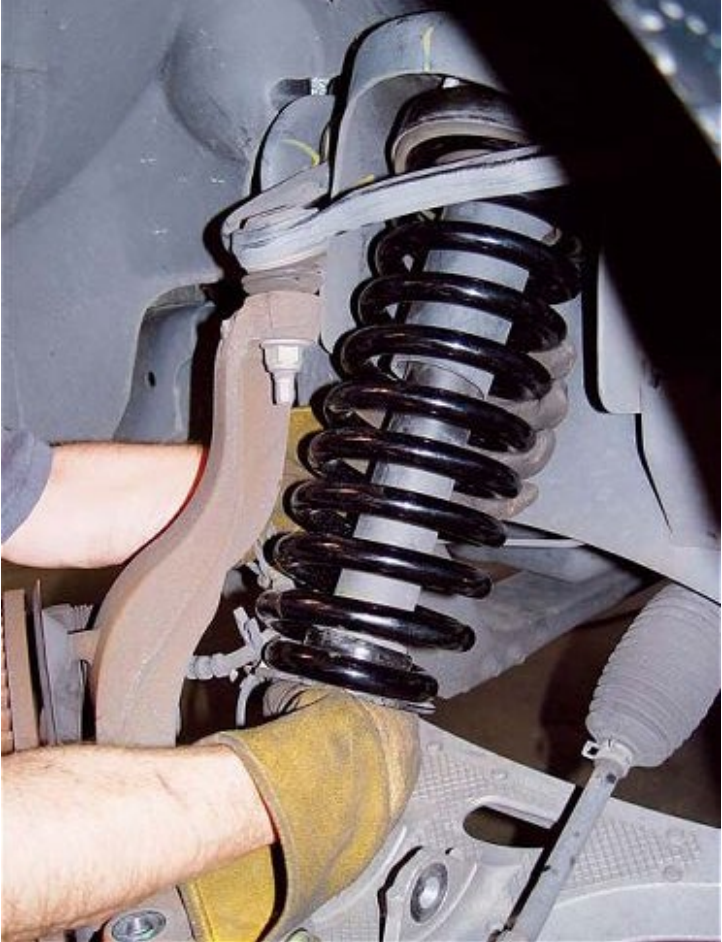
The front end will be 2 inches lower, once the weight of the truck is on the spring and strut.
