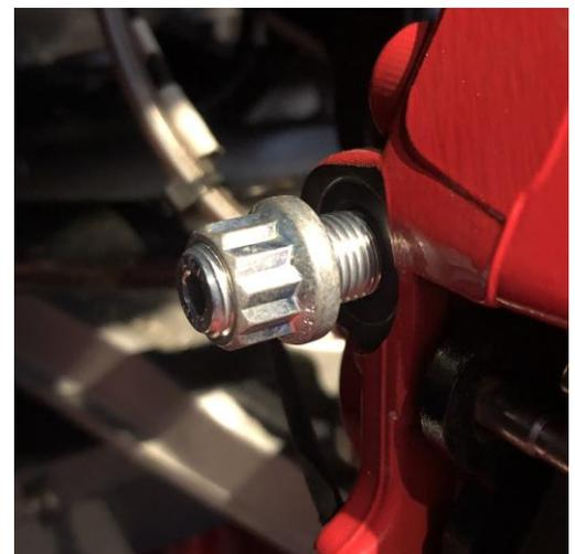
***Nut Installed before Tightening***
