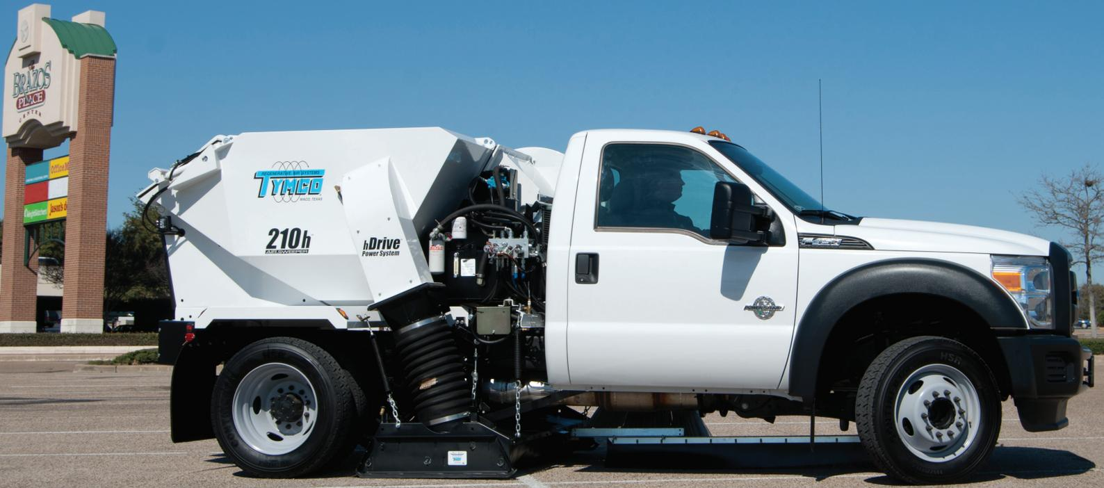
*The Model 210h® delivers great sweeping performance in a “single engine” class design. With the Ford Super Duty F-450, the Model 210h has a tight turning diameter of 44.2 feet, and overall height of 80.5 inches. The Ford F-350 turning diameter is 50.8 feet, and has an overall height of 78 inches, perfect for sweeping in parking garages.*
