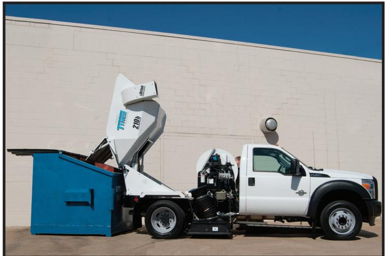
*With the Ford F-450, the Model 210h has a 62.5 inch dump height. (Most 6 yard containers are approximately 60 inches)*
