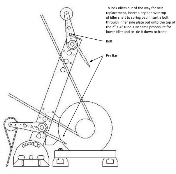
If you are unable to insert a bolt into tube to hold rear idler away from belt, use a rope or chain to tie it down to frame rail
