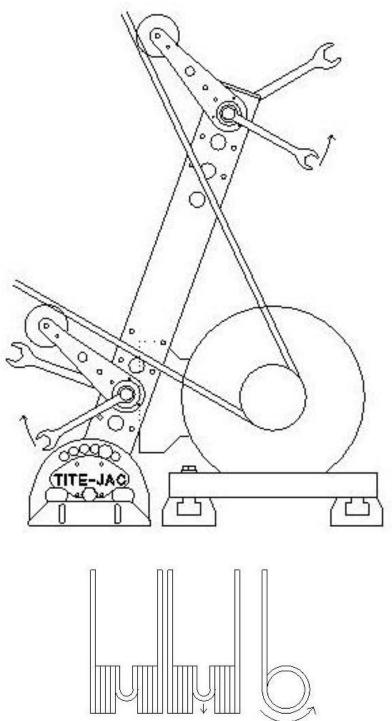
The spring tension must be adjusted in the direction indicated above. The spring must always wind tighter. If you tension the spring in the other direction, the spring will start to unwind and fail prematurely. These springs are the pickup tines from a New Holland combine and can be purchased at any agricultural implement dealer.
