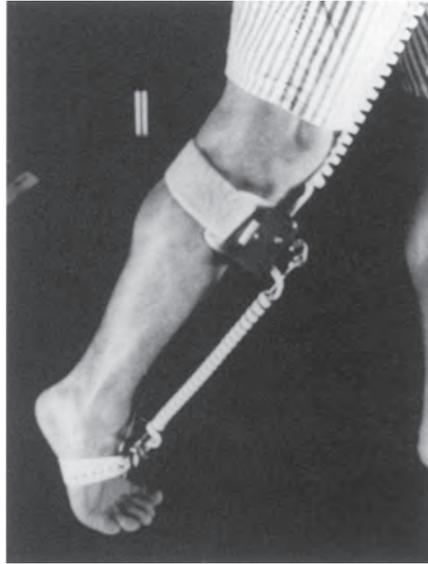
**Fig. 48** Electrogoniometer to measure foot and ankle motion.
