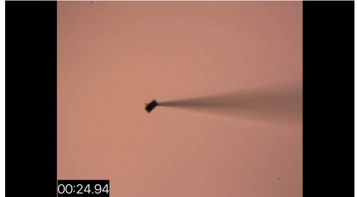
Pick of a specimen attached to a glass probe.
