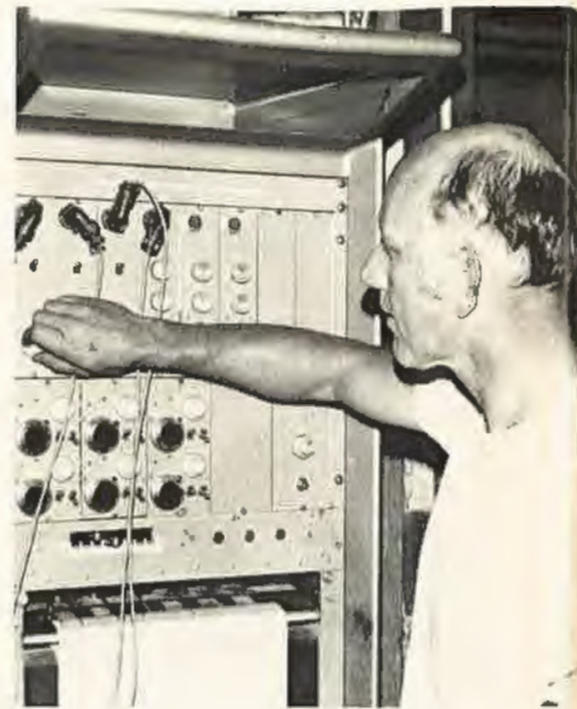
Left: Jim Ploen measures the time of relaxation of back muscles from the EMG records. Above: Dick Phillips adjusts the gain on the pen recorder.
