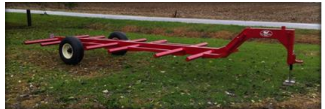
Arched tongue option, designed to work in tandem with C2200 Bale Spear/Trailer Mover. Arched tongue allows spears to clear when turning.
