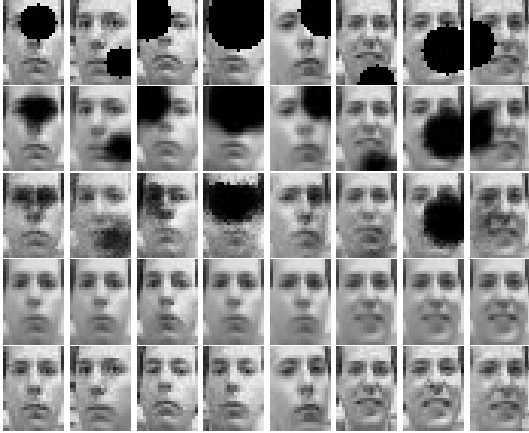
Figure 2: Visualization of recovery results on Frey face data. 1179 of the 1965 images (60%) were corrupted by a randomly positioned dark circle mark with random radius. Each column corresponds to a different database image. Row 1: Original contaminated samples. Row 2: Reconstructed images using RPCA. Row 3: Reconstructed images using an iC-VAE (no recycling). Row 4: Reconstructed image from an RiC-VAE( N=2, M=2 ). Row 5: Clean ground truth data without contamination.
