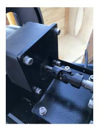
Loosen the 4 bolts that hold motor to mount and loosen couple set screws or bolts then remove motor and replace coupler. Next reassemble
