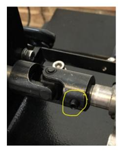
Can be replaced with with Heavy-Duty bolts with locking Nut. You can also grease coupler at joint
