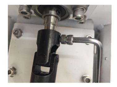
If you need to replace coupler you will need to loosen motor from motor mount and loosen the bolts or set screws on coupler to remove it:
