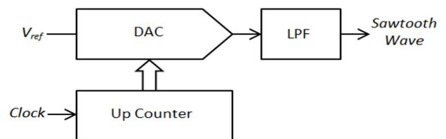
Fig 1: Basic digital saw tooth generator
