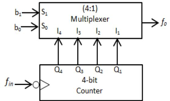
Fig 5: Programmable frequency divider
