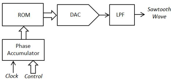
Fig 3: DDS based sawtooth generator
