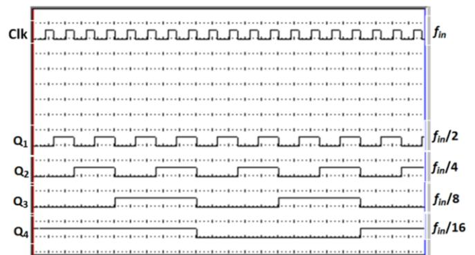
Fig 6: Data bits generated by counter
