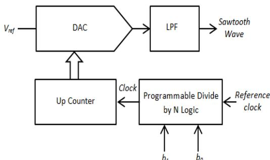
Fig 4: Proposed programmable sawtooth generator
