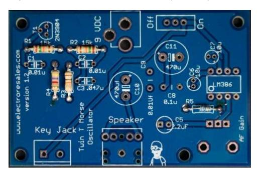
Stage 2 – Insert non polarized capacitors (C1,C2,C3,C8 & C9) – compare to this picture, orientation is not important
