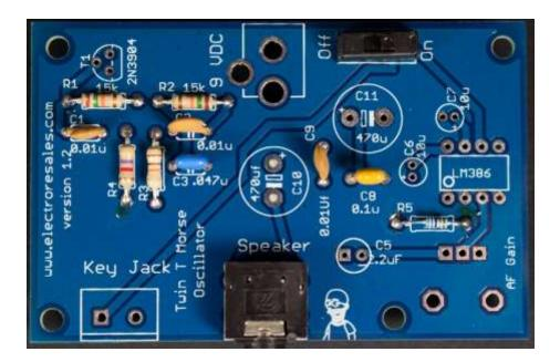
Stage 4 - At this step, add polarized capacitors C5, C6, C7,C10 & C11. Polarity is important here, make sure to align the component with the board markings for '+' or '-'
