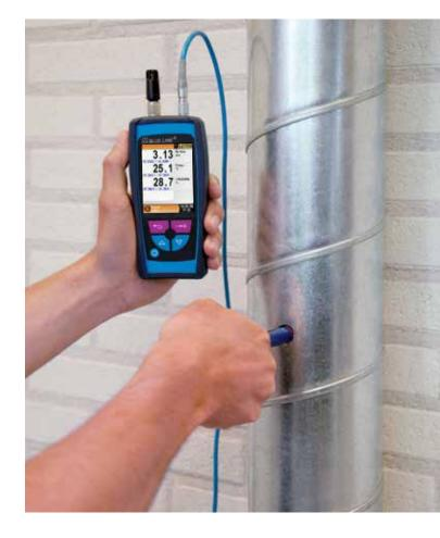
The BlueAir ST provides minimum, maximum and average values. The amount of air can be calculated by entering the dimensions of the ventilation duct. The device can be optionally equipped with a MicroSD card to store the measured values. A data logger function for automatic storage of measured values with adjustable frequency from 0 to 999 seconds is another possibility of the BlueAir ST. The device is equipped with Bluetooth ® Smart communication.
