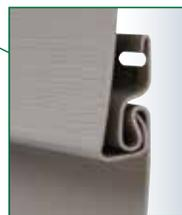
The heavy duty extended return leg snaps tightly into the **TitanBar** Reinforced Nail Hem which is double the thickness of the siding panel under the nail head, for an installation that's solid, secure and protects against panel blow off in adverse weather conditions.
