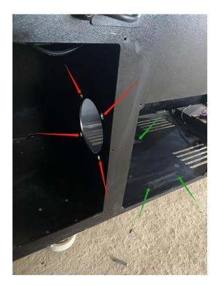
Here are 8 holes which are used to hold the cooling fan. 4 on the side, the other 4 on the base plate.
