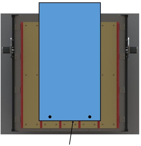
Place stock on the pins and clamp it down. You design should be broken into short enough parts that they can overlap.
