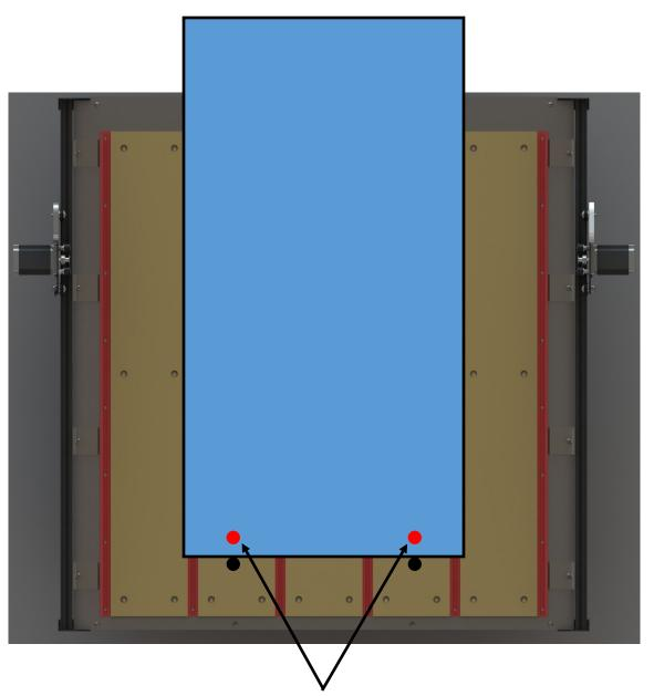
Then, bump the stock against the pins, clamp it down, and have the machine drill the same 2 holes in the leading edge of the stock. They should be fairly tight on the dowel pin diameter but still be able to be removed off the pins.
