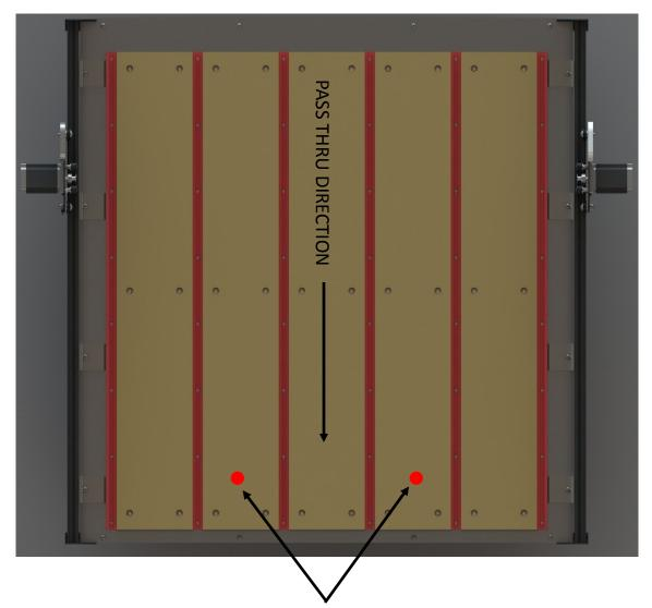
First, have the machine drill 2 holes in the waste board or a underlayment. The holes should be wider than any design you plan on carving. They should be very tight on the dowel pins going into them. These should be in known locations from home so you can start your design correctly.
